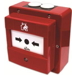
The Waterproof Addressable Manual Call Point has been designed to operate on a loop of intelligent fire detection devices and when activated interrupts the polling cycle for a very fast response. Available with and without isolator. It is intended for outdoor applications or areas where water ingress or high humidity is a problem.
