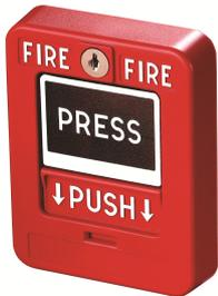
The Dual Action Addressable Manual Pull Station features translucent plastic at the centre, allowing visibility of an internal LED that indicates alarm condition and polling status. The unit is addressable using a DIP switch protected within the pull station. The pull station may be flush mounted on a single gang work box or use an optional back cover (56000-006).
